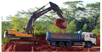
Chye Joo Construction became the first in the local industry to acquire the Volvo Tridem trucks, purchasing 25 units in October 2012. Each Volvo Tridem truck is able to carry a maximum 19 tonnage of load per trip, a 15 percent increase in payload compared to the regular 6x4, 10-wheeler tipper trucks.
