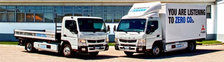
The new Fuso Canter E-Cell runs emission-free and almost silently has now been released for customer trials.
