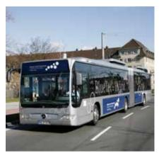
hub motors and the world's largest lithium-ion battery for automotive use. This battery stores the electrical energy from the diesel generator and that recovered by the braking system.
