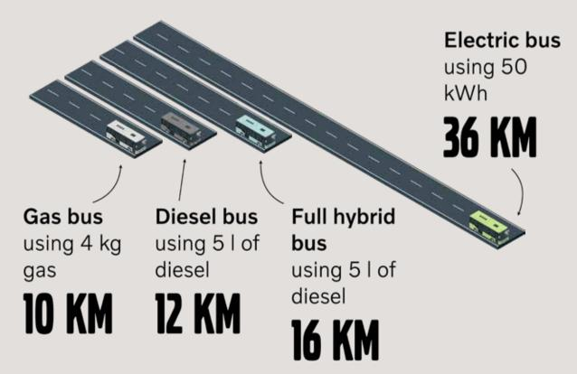
The calculation is based on tank-to-wheel energy consumption. Energy value of different types of fuel has been converted to kWh, where 4kg CNG = 51 diesel = 50 kWh electricity. Conventional diesel is used as a benchmark (100%) to compare results.
