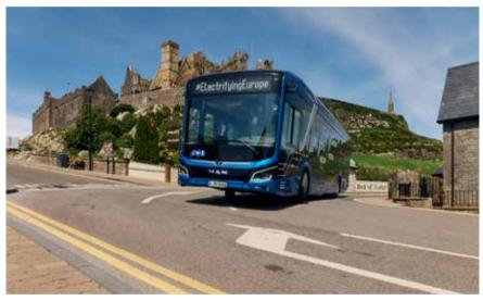
by six lithium-ion battery packs (capacity 480 kWh) on the roof of the eBus. Recharging was carried out after each daily stage; no intermediate charging was necessary.
