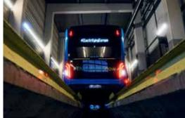
Total values of the MAN eBus Tour: Total distance 2 448.8 km Total energy consumption 1 763.7 kWh Total average speed 41.0 km/h Total recuperation rate 20.8 percent Daily values of the individual tour stages:
